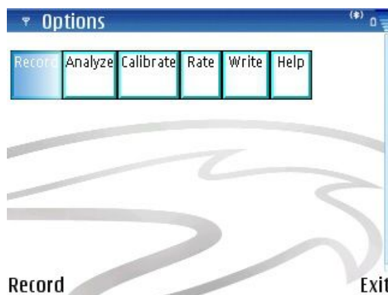
Figure 8. Menu options: Record records acceleration, Analyze acceleration. Calibrate calibrates the Wiimote accelerometers, Rate sets parameters for data collection and Write saves the data to a cell phone file.
